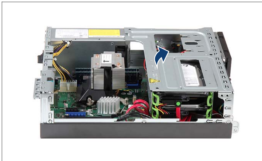
Figure 7: Opening the front cage
